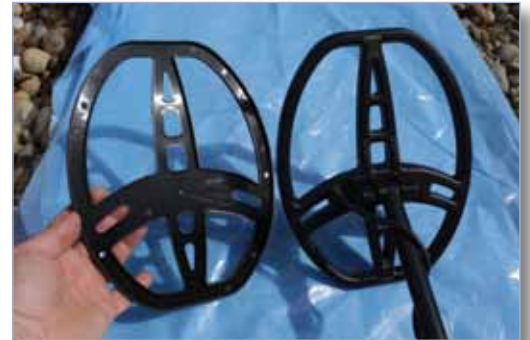
Fig.2. The coil and scuff cover.
