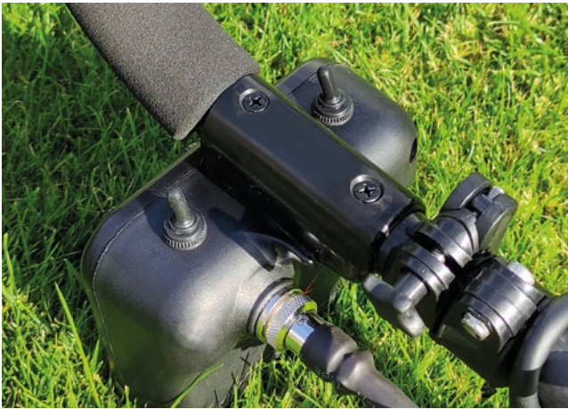
Fig.7. Both left and right handed toggle switches.
