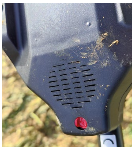
Fig.17. The rear speaker socket which ideally needs a cover.
