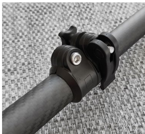
Fig.3. Carbon fibre shafts and adjustable camlocks.
