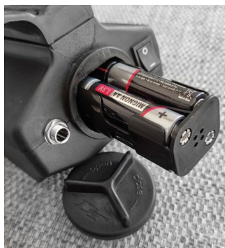
Fig.16. The 8 x AA battery compartment, power button and headphone socket.
