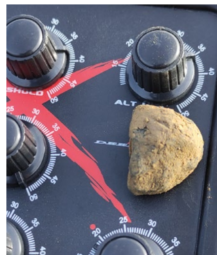
Fig.15. The Vista X likes coke but this was easily discriminated out with the Alt discrimination.
