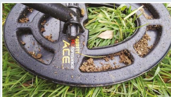
Fig.16. Coil cover full of soil.
