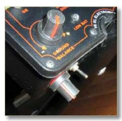
Fig.2. Frequency Adjust control and the Turbo Boost switch.
