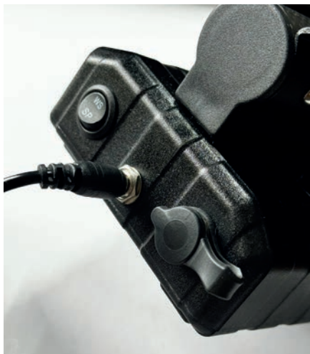
Fig.5. The rechargeable battery and switch to change between external speaker and wireless headphones.
