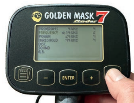
Fig.12. The four frequencies available with the option of up to 8 levels of frequency shift on each programme to remove any EMI.
