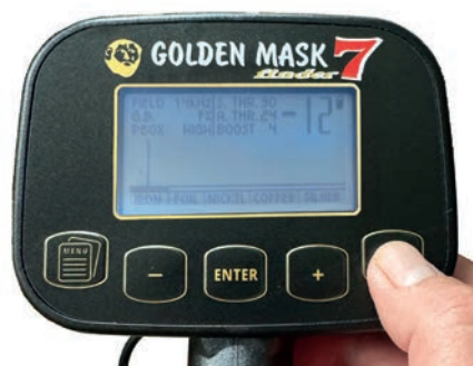
Fig.14. The Spectrum VDI display bar and negative target ID clearly depicting iron.
