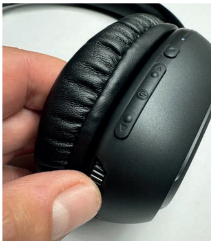
Fig.6. The exceptionally comfortable headphones with scroll wheel to adjust the volume.
