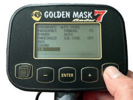
Fig.13. The wide range of Ground Balance options including the new FX Mode on the GM7.
