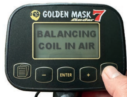
Fig.9. Automatic calibration of the GM7 on start-up.
