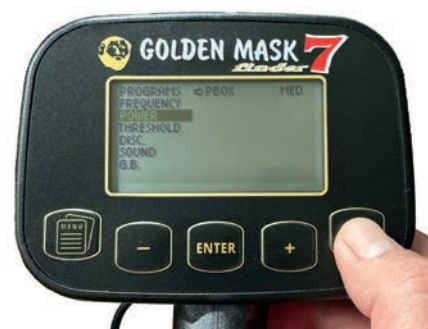
Fig.15. One of my favourite features the 'PBOX' option to increase power from the machine to the coil.
