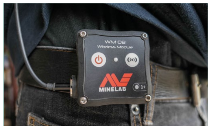
Fig.3. WM08 wireless module, which clips onto a belt.
