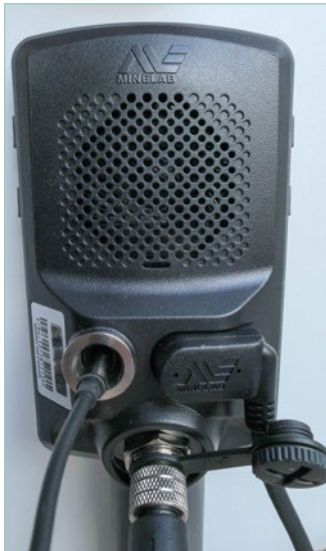
Fig.4. The back of the console showing headphone socket and charging socket.
