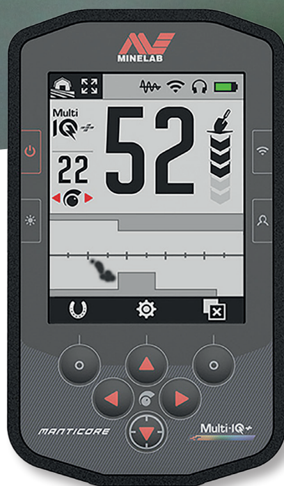
Fig.9. Example of targets on the 2D display in heavy alkaline soils.
