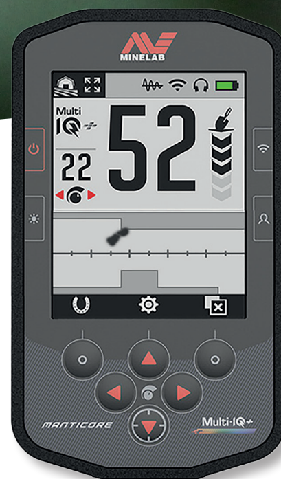
Fig.10. Example of the 2D display in heavy iron sites or with magnetic properties.
