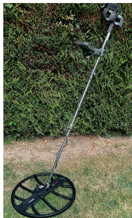
Fig.1. The MythTek 18-inch coil fitted to my Minelab Manticore on the day of delivery.
