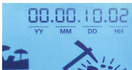
Fig.7. No more 'used once' if not true. You can now see how many hours the Legend has been used to detect!
