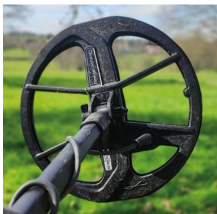
Fig.2. The carbon fibre shaft and coil.
