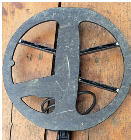
Fig.9. The coil cover does not quite protect against dirt and soil ingress.
