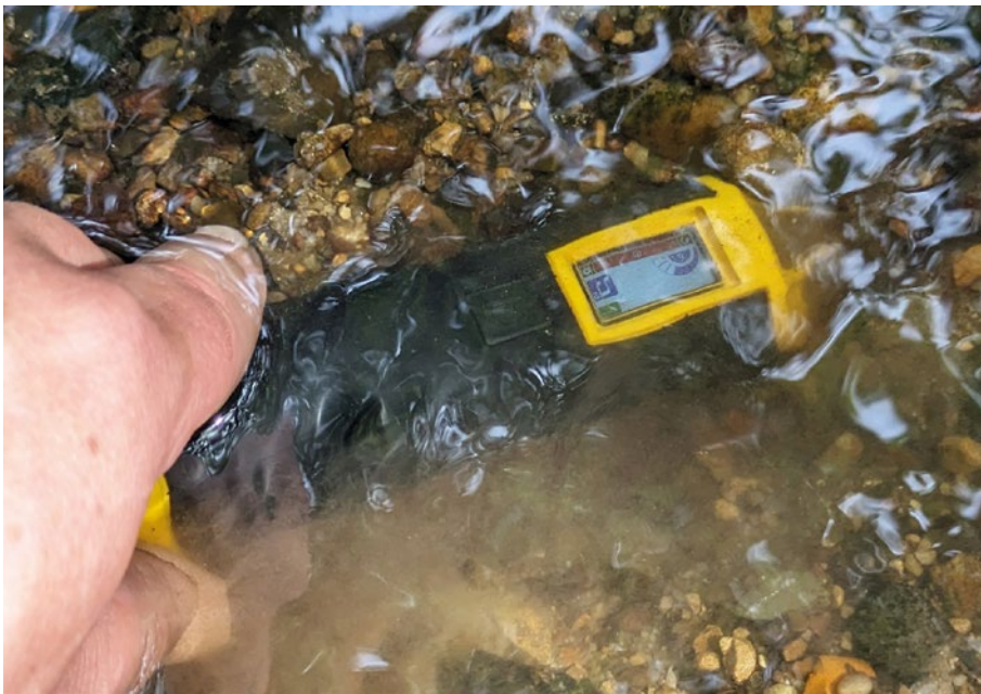
Fig.8. Although waterproof up to 3 metres, the AccuPoint easily handled over an hour submerged in a stream.
