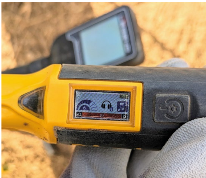
Fig.3. The AccuPoint screen and single button after pairing to headphones.
