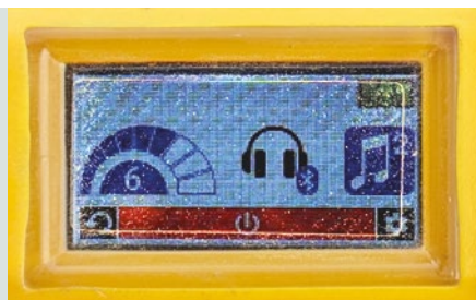
Fig.3. The AccuPoint screen and single button after pairing to headphones.
