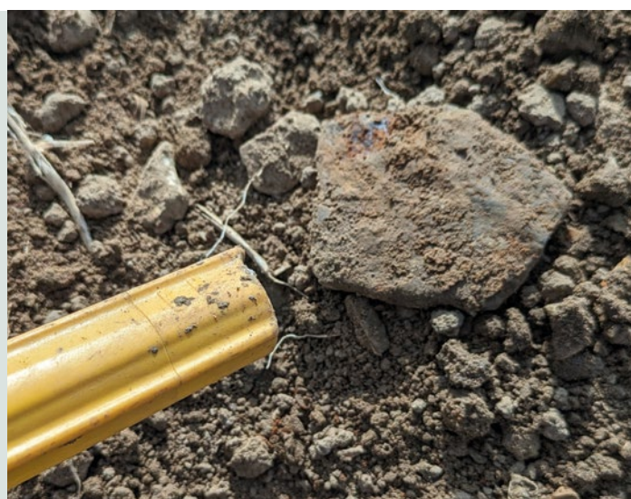
Fig. 7. Testing out the ferrous tone on the AccuPoint.
