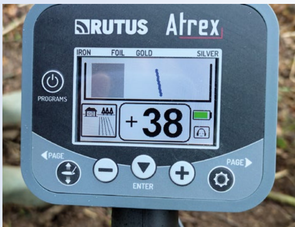
Fig.10. A semi straight line on the hodograph display of the Atrex in Basic Mode, showing a nice target.
