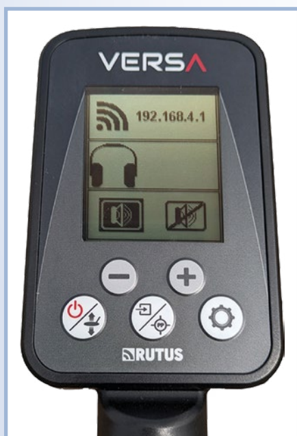
Fig.11. Simple 'no leads' software update on the Versa.
