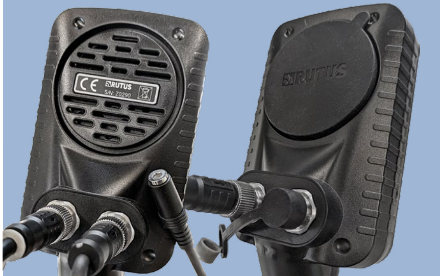
Fig.6. Back of the control box without and with underwater protection.
