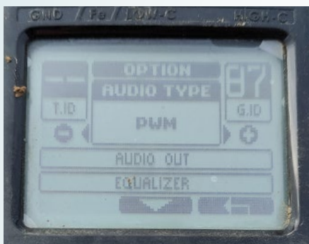
Fig.13. The original PWM XP harmonics sound option.
