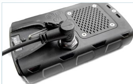
Fig.6. Plastic plug on underside of control box.
