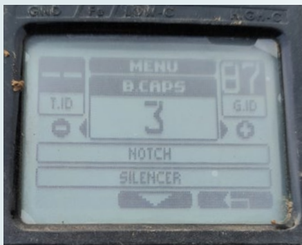
Fig.12. The new bottle cap rejection settings.
