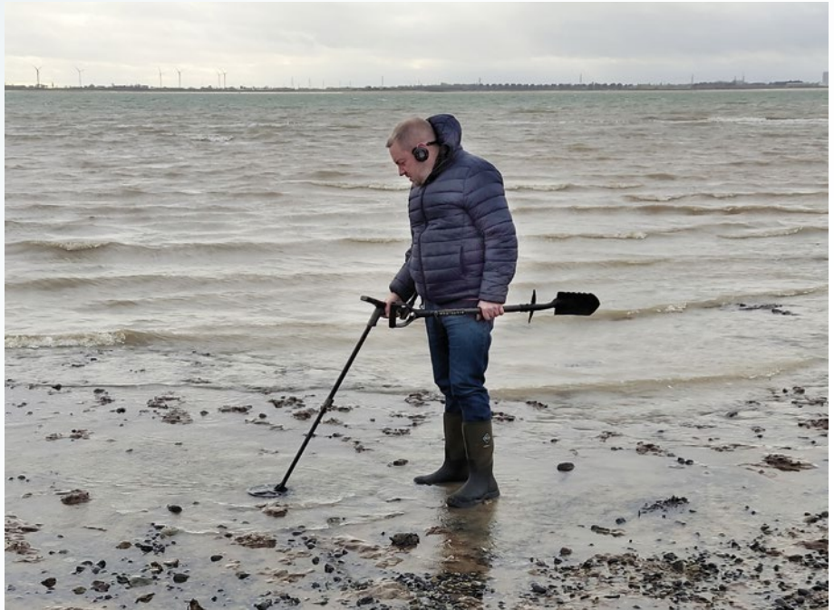
Fig.20. No problems with the coil submersed in saltwater.
