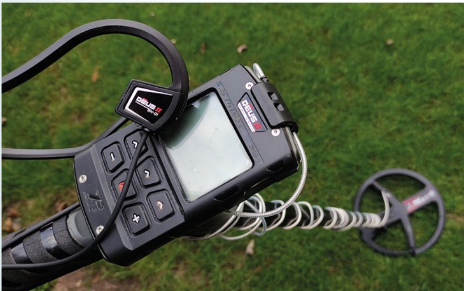
Fig.7. The Deus diving configuration with bone-conduction headphones.
