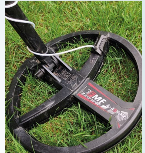
Fig.8. Deus II coil amplifier in place.
